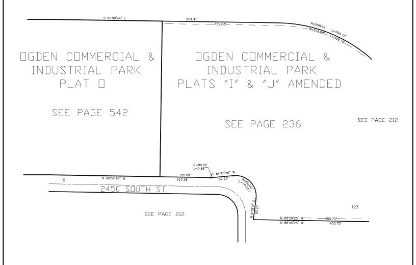
10' UTILITY & DRAINAGE EASEMENTS EACH SIDE OF PROPERTY LINES AS INDICATED BY DASHED LINES EXCEPT AS OTHERWISE SHOWN.
